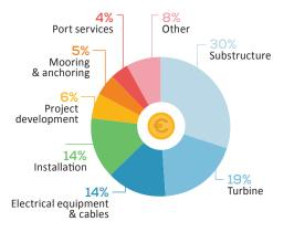
CAPEX of a pre-commercial floating offshore wind farm Source: ETIPWind
